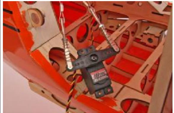
39. It is easiest to complete the cable setup at the servo end prior to installing the servo in the fuselage.
