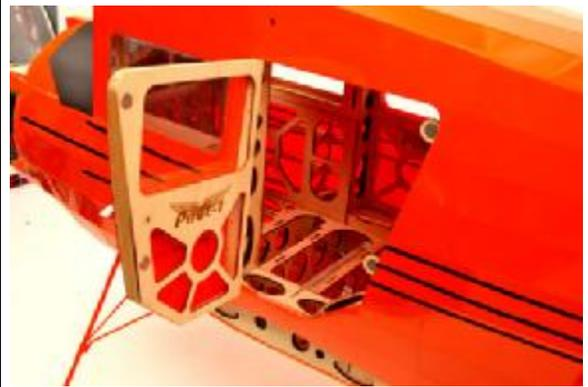
122. Locate your radio receiver on the floor of the cabin with easy access. 6" servo extensions on the 2 aileron channels of the receiver will make connecting the ailerons easier.
