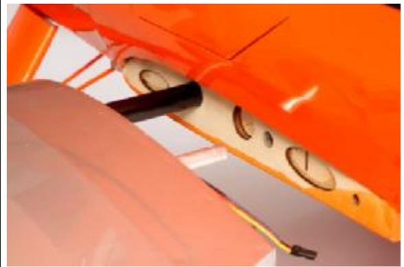
73. Locate the 4 hitch pins. The wing panels are held in place with these pins, no screws or bolts are required.
