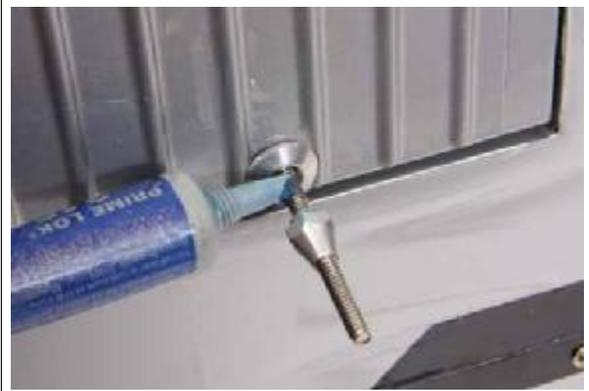
22. Screw nylon control horn linkage to the control horn. The distance from the bottom of the aileron to the center of the hole on the nylon part should be about 28mm (1-1/8").
