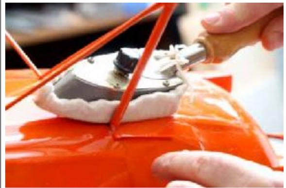
61. Using a covering iron with a sock on it, iron the covering into position.
