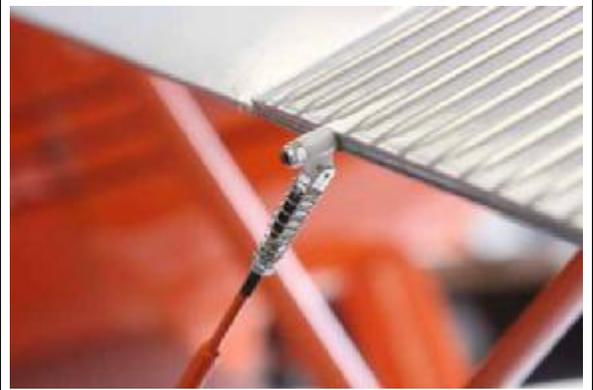
92. Locate the tail brace wires and solder on electrical ends as well as the 3-3mm allen head screws and 3mm nylock nuts.
