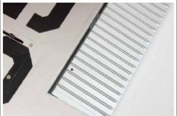
16. Deflect aileron upwards and repeat application for bottom of wing. Note very small gap between aileron and wing.
