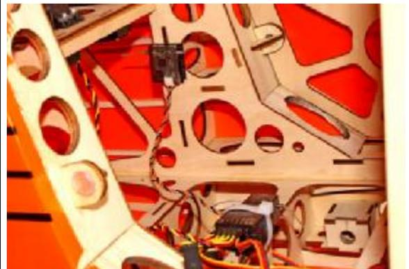
124. Flight batteries are installed in the inside of the motor box in the nose of the aircraft. You will need to build a platform on which to attach the batteries. The exact dimensions of this will be determined by your choice of batteries. Make sure that they are secure before flight.
