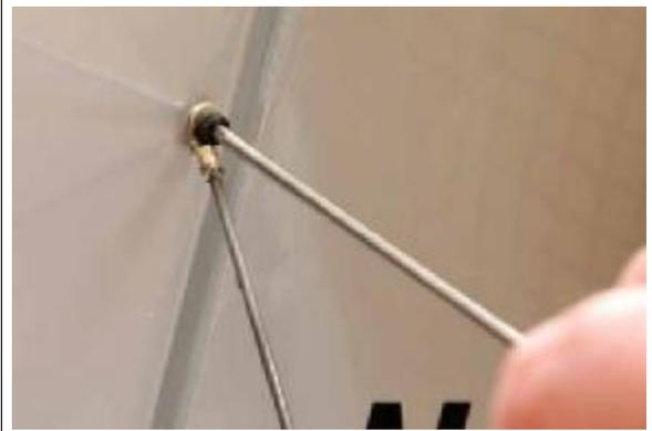
98. On the bottom brace wires solder the terminal so that a wood screw can be used to attach it to the fuselage. Pre-drill the fitting before installing the screws.
