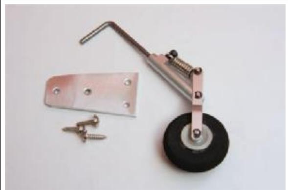
30. Mount the aluminum plate to the bottom of the fuselage with 3 screws. The bend in the aluminum plate goes down.
