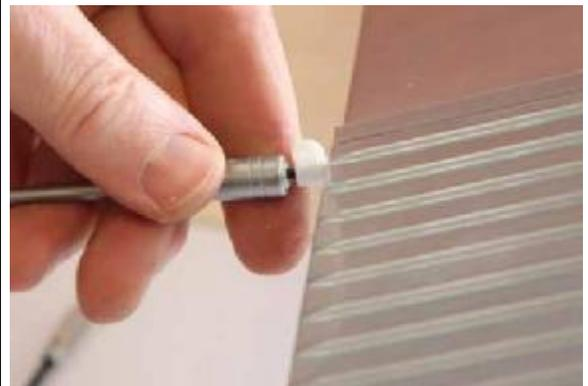
89. Install aileron inter connector celvis to the nylon part.
