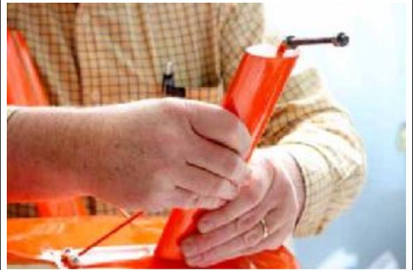
64. Insert balsa strips into the groove to finish the inside of the gear leg.
