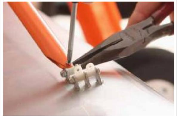
82. The N struts are 3 different lengths with the longest at the rear, the shortest in the middle (the diagonal) and the middle length strut at the front. The photo shows the upper connection of the N struts at the rear of the wing.
