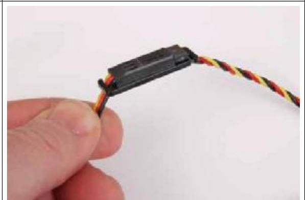
7. Slide the servo extension through the wing to the root.
