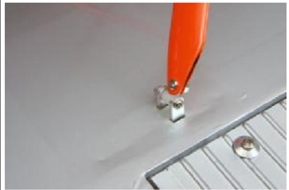
87. Locate the hardware for the aileron interconnection.
