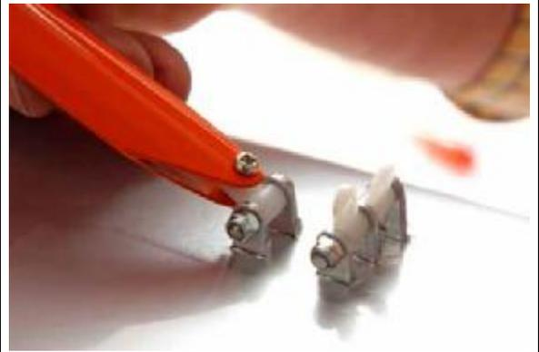
81. Hold the nut with a pair of needle nose pliers while you screw the Phillips head in place. Repeat at the upper end.
