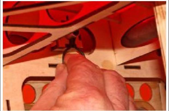
127. Unplug the aileron extensions from your receiver and slide the wings away from the side of the fuselage about 2-3".
