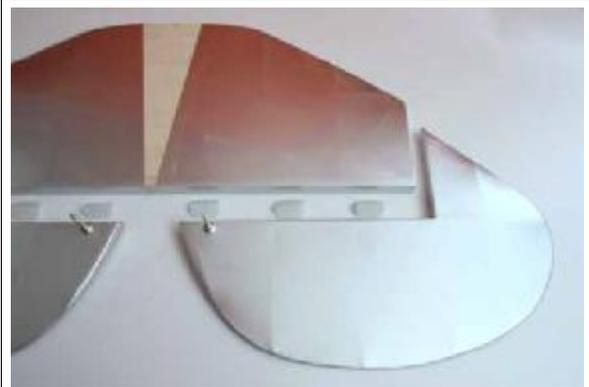
33. Prepare the vertical fin and rudder for installation. Install CA hinges in rudder and fin.
