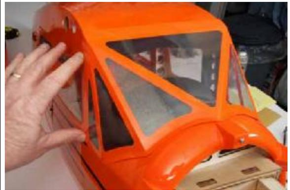
119. Access to the radio system and the batteries is through the operable doors.
