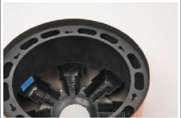
104. The cowl mounting ring is pre-installed at the factory. Installation is by placing the cowl over the cowl mount screws and rotating slightly in a counter-clockwise direction to hold in place.
