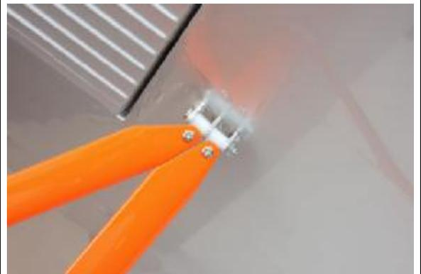
83. Photo shows the upper connection of the N strut at the front of the wing.
