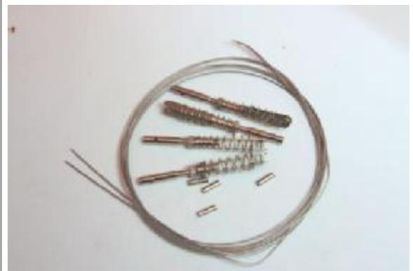
37. Thread the bare end of each cable into fuselage at rear. A tube is a pre-installed for you. Pull all but a few inches of cable to the front. Tape the rear of the cables so that they remain accessible.
