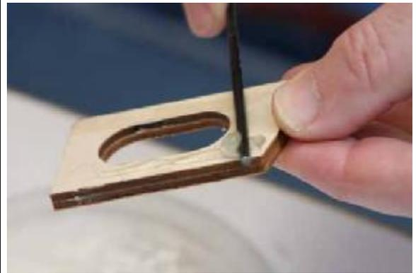
52. Insert glued filler in position. Have a small hammer handy to tap the block in place.
