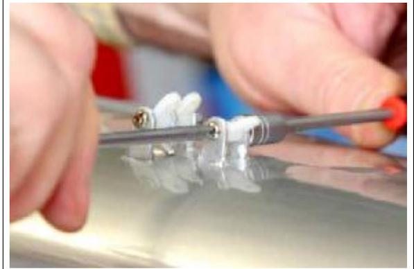
79. When all fittings are installed on the wings begin to install the struts with the long diagonal strut.
