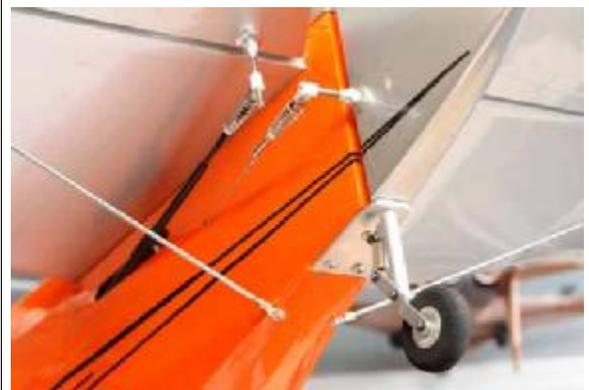
101. Bottom view of elevator pushrods, pull-pull rudder with tail wheel steering and the lower mount points for the tail brace wires.
