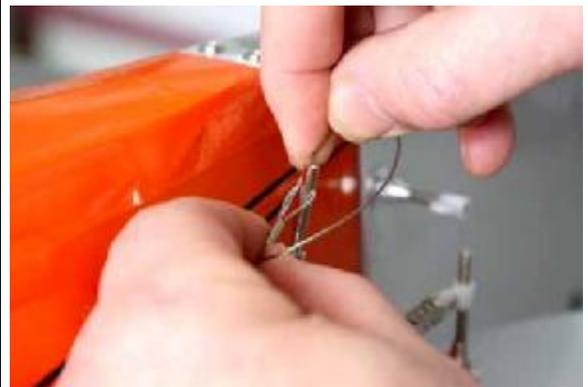
42. Install the pull-pull control horn through the rudder and center. Use thread locker to keep the unit tight.
