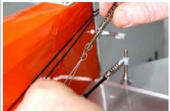
45. After you are satisfied that you have the cable lengths correct for centering your rudder, and that the servo is still in its neutral position, crimp the wire in position.
