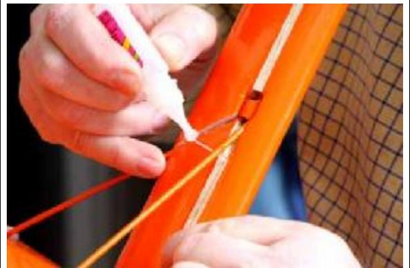
66. Cut lengths of orange covering to finish the interior of the gear legs. Iron one edge of the covering into position.
